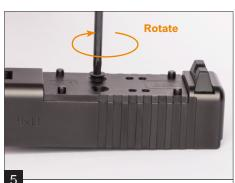
Tighten the 2 screws to fix the GLOCK MOS Adapter Plate on your GLOCK MOS Pistol. Screws should be tightened to a secure hold. (Attention: The set includes 1 additional replacement screw. It is not recommended to use these screws to fix the optical system itself.)
